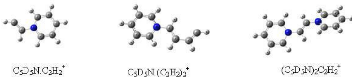
Figure 57. Proposed Structures of C_5D_5N.C_2H_2^+ ( m/z=110 ), C_5D_5N.(C_2H_2)_2^+ ( m/z=136 ), and (C_5D_5N)_2C_2H_2^+ ( m/z=194 ).
